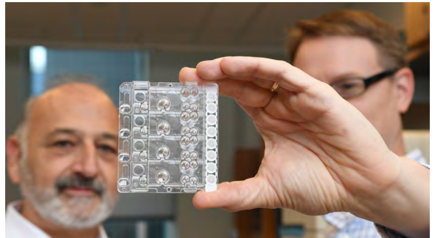
The COVID-19 MDx Assay is a biomolecular analyzer that can detect COVID-19 using genetic material from a respiratory sample. Credit: Nancy J. Parisi.
