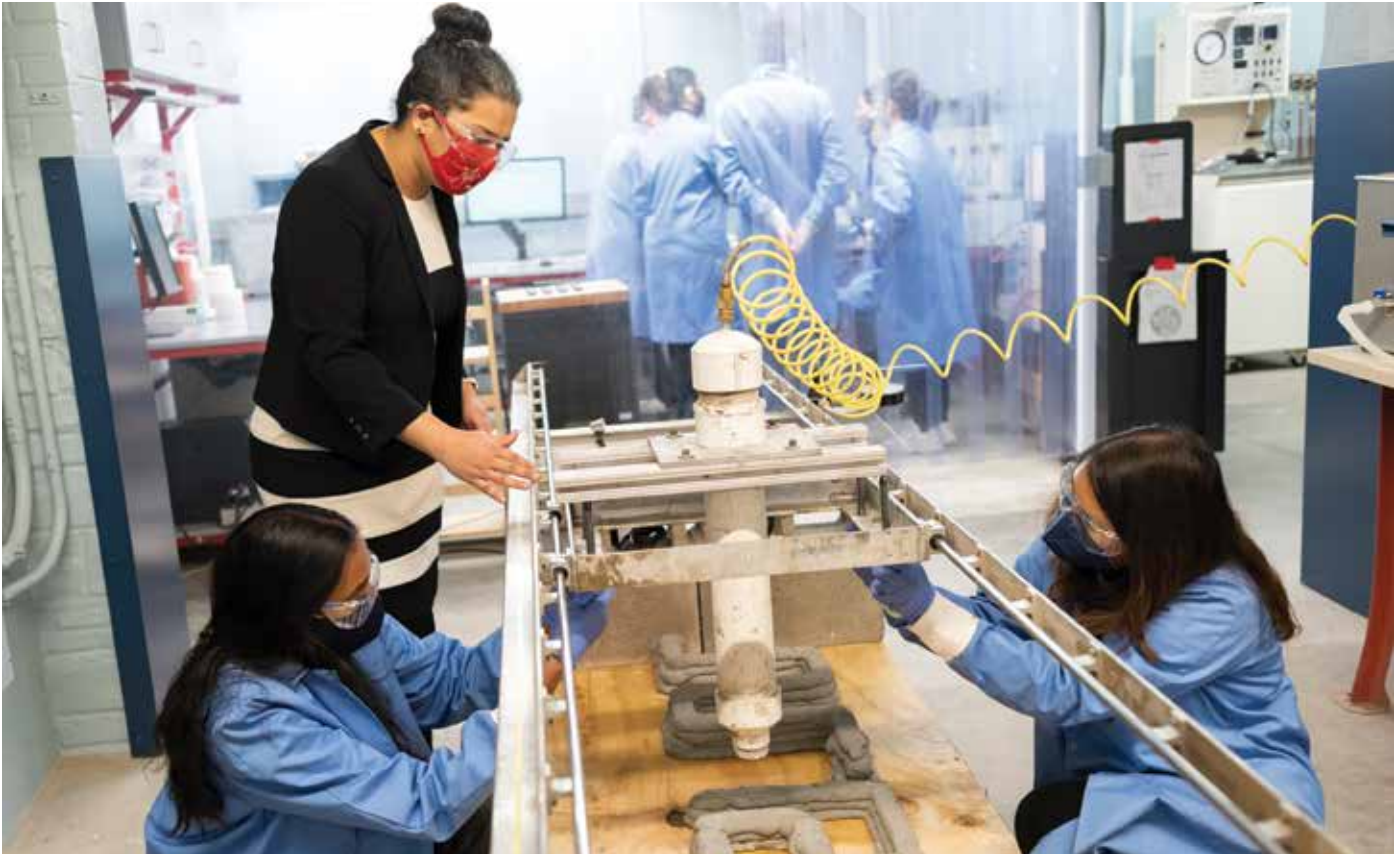
Assistant Professor Sriramya Nair (top left) and her students operate a 3D printer that deposits cementitious materials in the Bovay Laboratory Complex.
