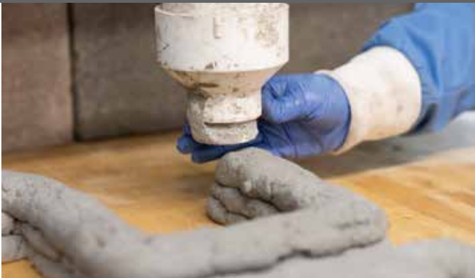
A cement mix is deposited from a 3D-printer head in the lab of Assistant Professor Sriramya Nair.
